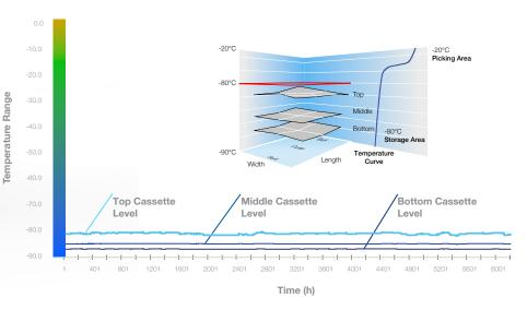
Two climate zones, one for active components at -20°C and another for passive elements at -80°C. Proven, stable horizontal temperature layers within the ULT storage area.
